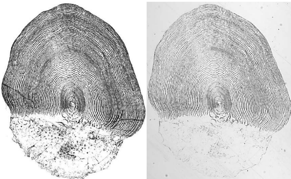
Figure 16. Figure on the left is from washed and not pressed 2SW (two-sea-winter) salmon scale and figure on the right is from the same washed but pressed scale.
